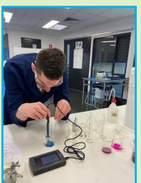
Jesse Amos is using the Vernier Data Logger (provided by Parents club) to determine the pH at which synthetic and natural indicators change colour or when the end point of a reaction can be determined, and in this case, of an acid base reaction.
