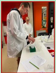
We looked at flame tests (which we had done before) and then what we really came for: the Atomic Absorption Spectroscopy. This measures the actual concentration of sodium ions (salt) in the water. We had a bit of trouble getting acceptable results for the standards we made up, but eventually we got there.
